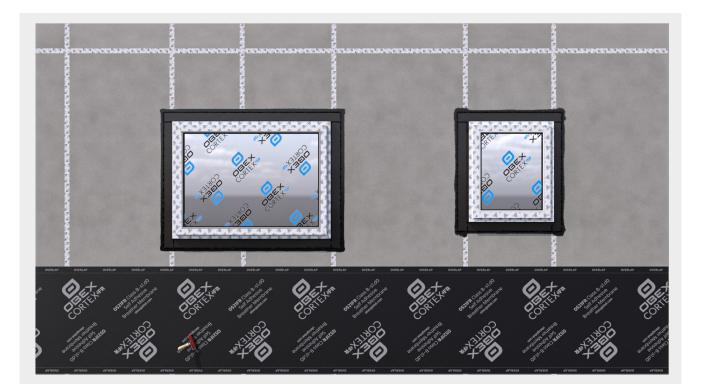
Remove the release liner and affix the lower half of the membrane, using the roller to ensure a good bond.
