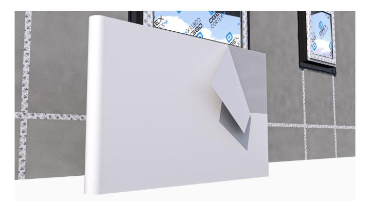
Peel back a section of the top release liner and apply the top corner of the membrane onto the substrate at the desired position. Start from the bottom and work upwards, ensuring that upper layers lap over lower layers.
