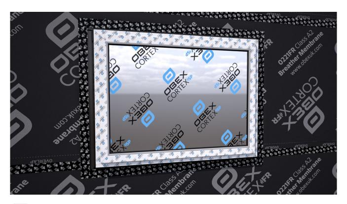
Finally, apply 0823FR over all edges of the breather membrane around windows, doors and any other penetrations. Start from the base and work to the top to ensure the tape is correctly lapped.
